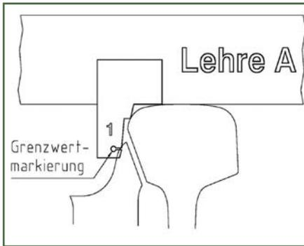
Figure 2, left, show an inspection of switch rail damage/wear (SBB). Table 1 is a summary of potential measurements in the switch area.
