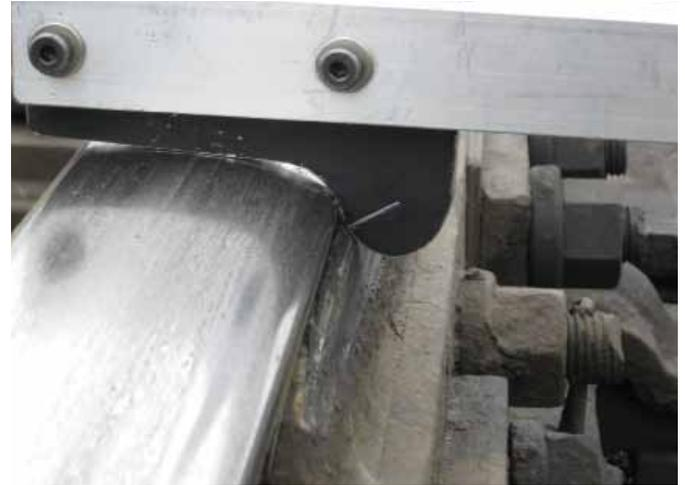
Left, Figure 4, new AAR1B Wheel Profile Gauge in bottom measurement position. Severely worn AAR 1B wheel profile in top (inactive) position. Figure 5, contact below 60-degree mark on new AAR 1 B Wheel Flange Gauge.
