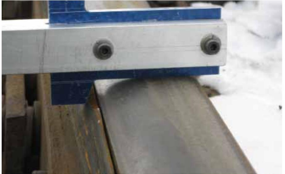
files (both narrow and wide flange) and measured switch point profiles. This included analysis of the location of the gauge point of wheel (where radius reverses on wheel flange), where there is the greatest potential for wheel climb. As illustrated in Figure 1, for the AAR 1B narrow flange wheel, the
